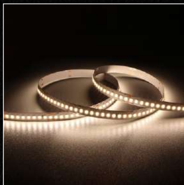
GS-2835-180LED-12V/24V WATTAGE :-15W CCT :-3000K/4000K/5700K
